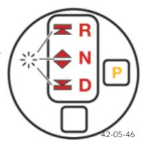
This display is illuminated when the transmission is in the mechanical or electrical emergency operation and the CAN communication is not functional.
